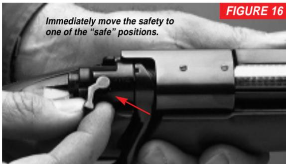
3. Push the bolt fully forward, positioning a new cartridge from the magazine into the chamber. Lock the bolt by moving the bolt handle (knob) fully down. Your rifle is again cocked and ready to fire. Immediately put the safety in the middle or rear “on safe” positions until you are ready to fire again (See Figure 16).
