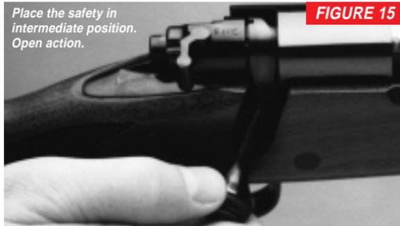
**IMPORTANT— ALWAYS VISUALLY CHECK AND KNOW FOR SURE THAT YOUR RIFLE IS NOT LOADED. DO THIS BY LOOKING DIRECTLY INTO THE CHAMBER AND MAGAZINE WITH THE ACTION OPEN AND BOLT FULLY TO THE REAR.**
